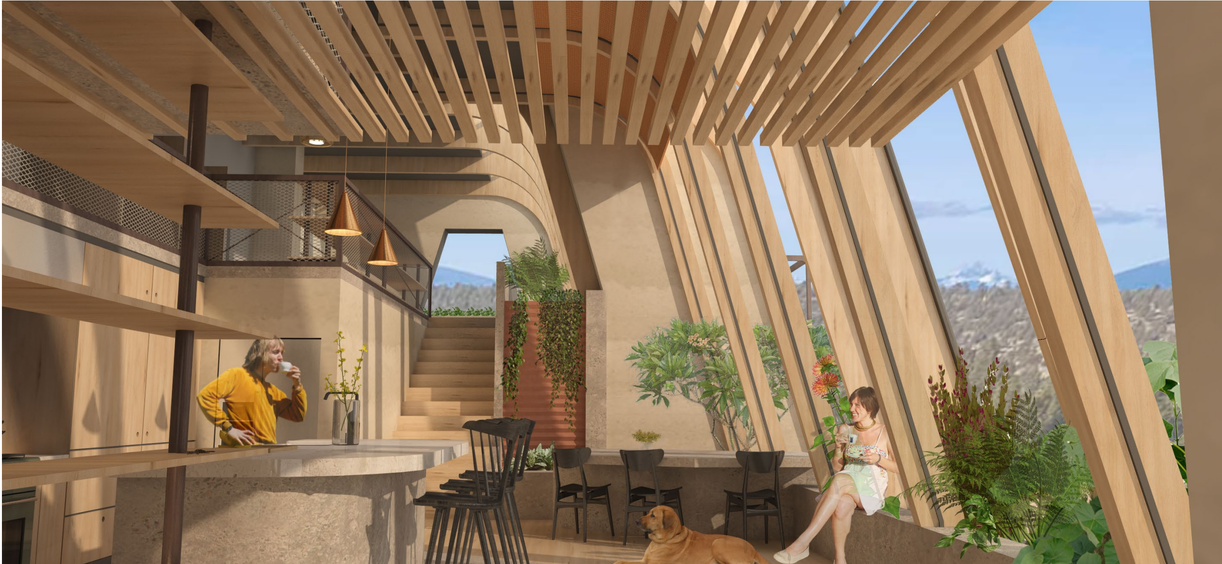
Southern sun rays kiss the faces of rammed earth walls and inhabitants, fueling passive heating and warm moods. Interior planters grow supplemental produce and herbs, while cleaning gray water. This process is highlighted by a water feature flowing from the second floor to the second.
